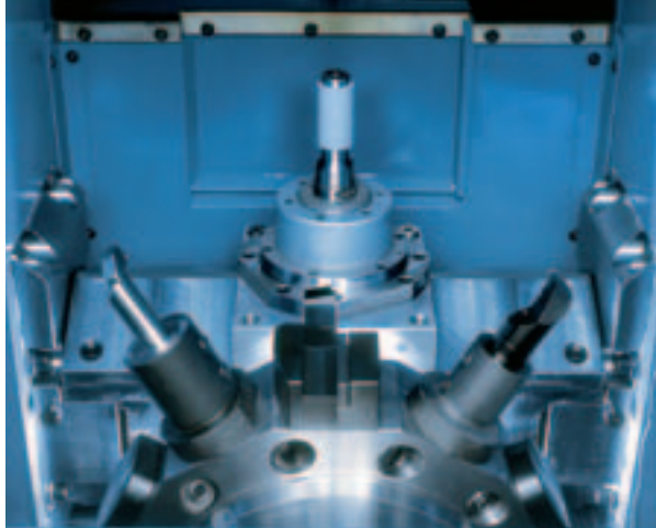
Disc-type turret for 12 turning tools and one fixed spindle for internal grinding work.
