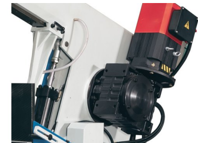
Infinitely variable belt speed, servo motor driven
