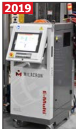
MILACRON MOLDMASTERS EM3-250SC-38 E-MULTI all electric servo driven auxiliary plastic injection unit
