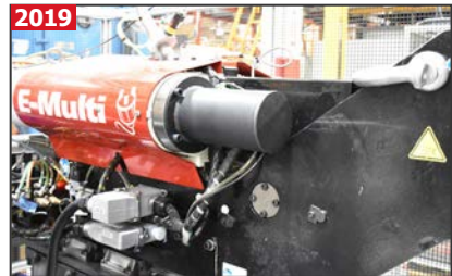
MILACRON MOLDMASTERS EM3-250SC-38 E-MULTI all electric servo driven auxiliary plastic injection unit
