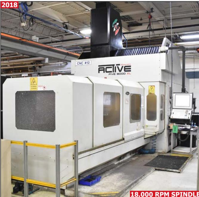
OMV PARPAS ACTIVE FIVE XL LINEAR 3000 high speed 5-axis bridge type CNC vertical machining center
