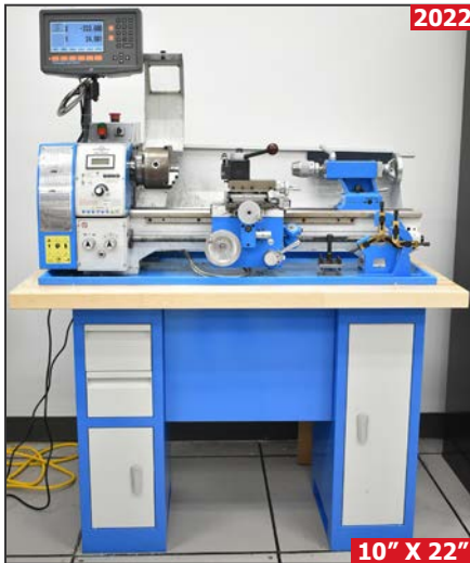
PRECISION MATTHEWS PM-1022V benchtop tool room lathe
