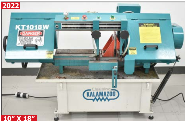
CLAUSING-KALAMAZOO KT1018W conventional horizontal band saw
