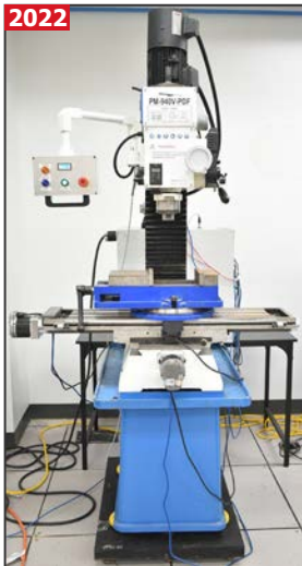
PRECISION MATTHEWS PM-940V-PDF vertical milling machine
