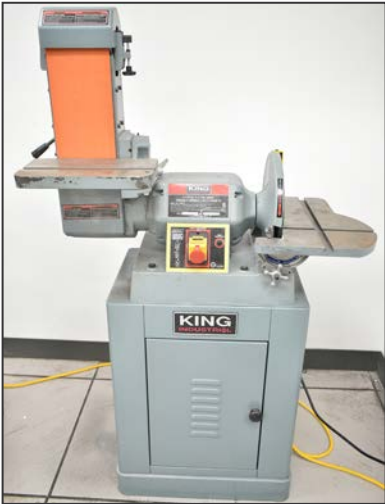
KING INDUSTRIAL KC-790FX floor-type combination sander
