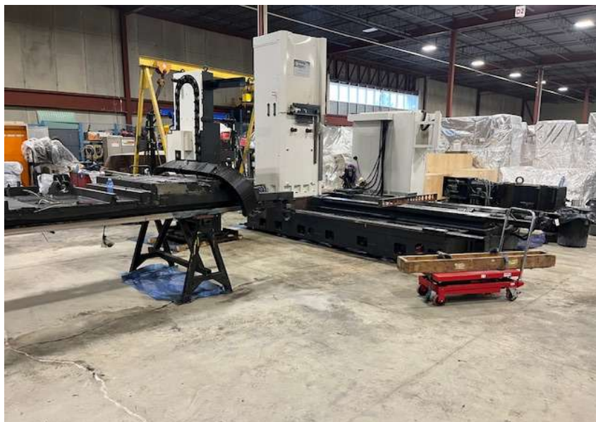
Main Bed, Z axis Saddle and Table Saddle after turcite is removed
