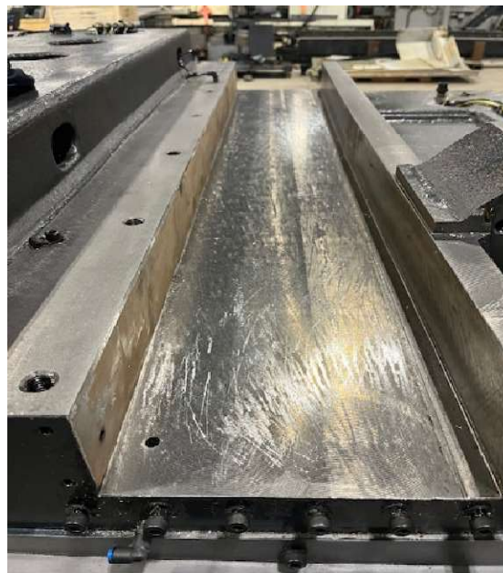
Main Bed, Z axis Saddle and Table Saddle after turcite is removed
