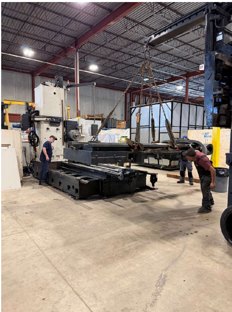
Re-Installing Z axis saddle
