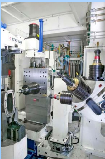
T2 TWIN SPINDLE T2 LATHE TWIN or SINGLE SPINDLE Y-AXIS +/- 50MM
