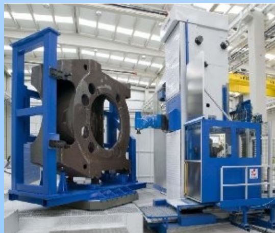
M2-5-AXIS TRAVELS: 29.5 X 25.5 X 19.6 20,000-RPM SPINDLE
