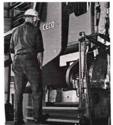
FIG. 13 SAFETY TREADLE AND COVER
