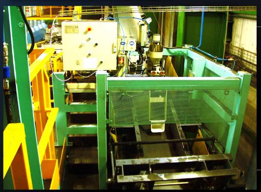
The SPACE GSM Green Sand Laboratory is the ideal equipment to manage the irregular quality of return green sand. By measuring the on line characteristics of the prepared sand, such as compactibility, compression, green shear, temperature and moisture, it can adjust water and dry additions, automatically, in real time.
