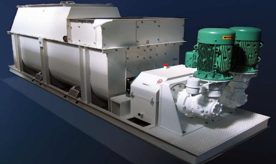
THE SPACE MU Pre Mixer Homgeniser unit is used for the addition of water and additives to green sand prior to the bulk sand storage. This equipment not only promotes the spontaneous development of the bentonite but also conditions the sand in a uniform manner, ready for final mixing.
