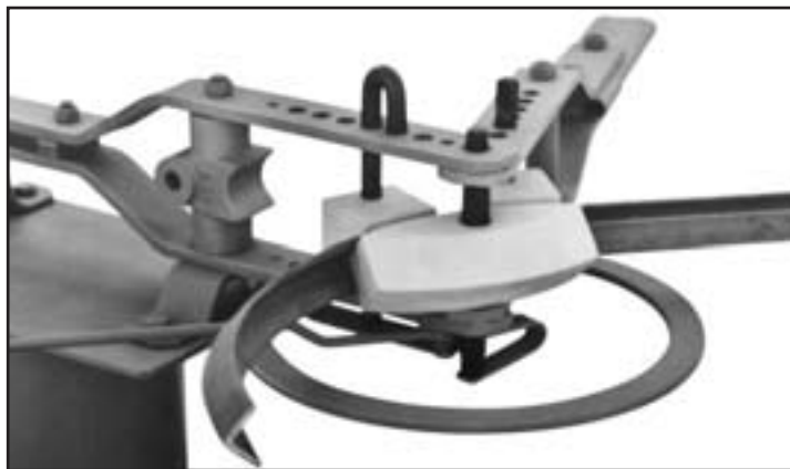
20B10 Form Die with 42990 Back Block/Draw Block Set bending Angle Iron with the "Heel Out"
