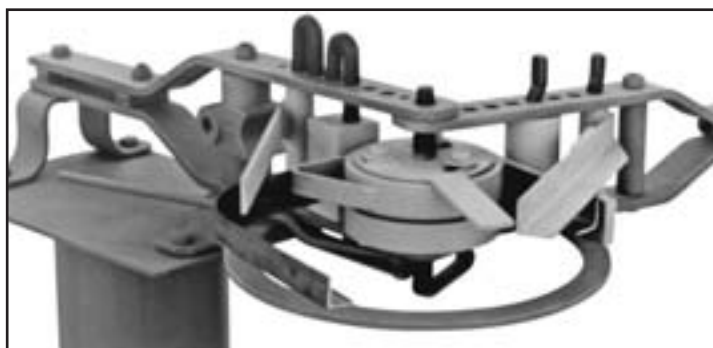
102B Form Die with attached Hold-Down Arms bending wide U-bend in Angle Iron, “Leg-In”, to a 2-3/4" radius
