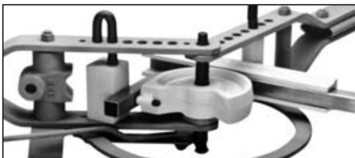
11B Square Block used as backing block with 37894 Dowel Pin inserted in Form Die to secure the stock
