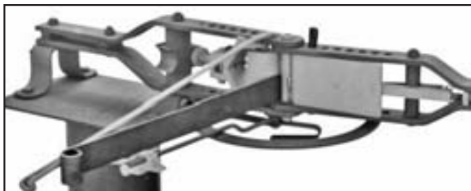
2B Roller & Shoe, mounted on Main Frame Arm (left), and 4B Gripping Blade, mounted on Swing Arm (right), grab and hold Flat stock while bending it around 5B Pin of the desired diameter, forming a closed Eye. 1B Extension Rod Support holds stock steady.
