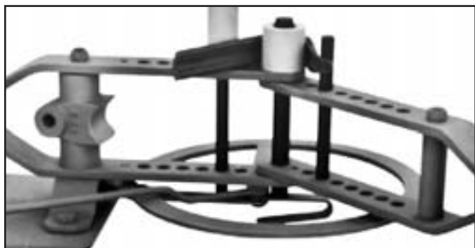
Completing Lambs Tongue using 20B7 Steel Roller
