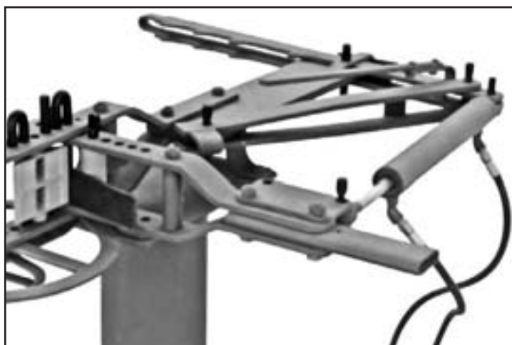
Sharp Square Bending Block forms sharp square bend on wide flat stock with hydraulic assist
