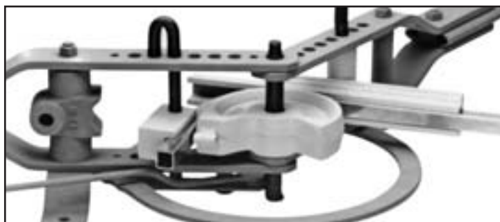
103B Square Tube 180° Die Set (Form Die, Back Block, Draw Block) bending a 4" radius in 3/4" Square Tube
