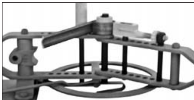
16B2 Wide-Nose Bending Dog bending Volute around 20B7 Steel Roller
