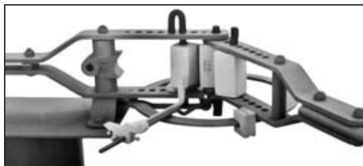
8B Cam Die (2") and 11B Square Blocks bend 'U'-Bolt in Round Stock to a predetermined point set by the 27B Circle Stop Gauge
