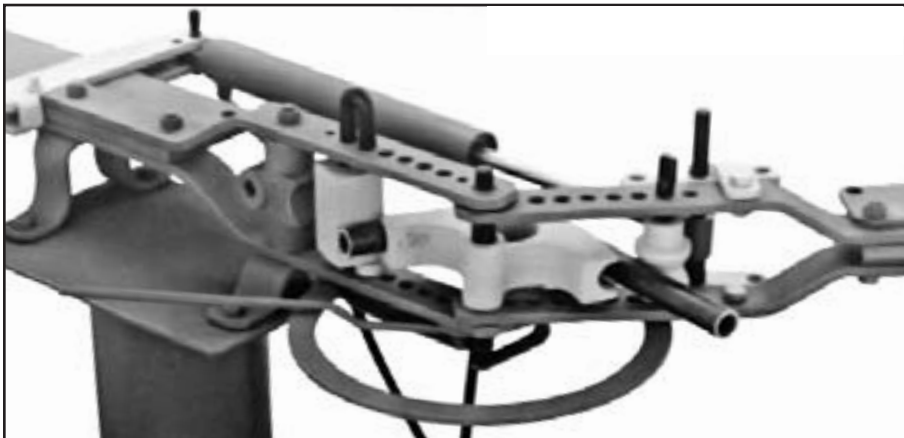
Hydraulic Cylinder attached using H55 90° "One-Stroke" Hydraulic Cylinder Mount. 44B Rigid Conduit 90° Die shown bending 1" Pipe to 90° with a single stroke
