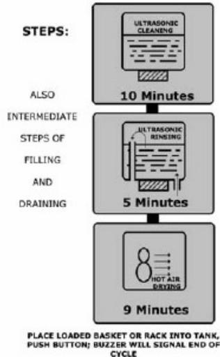
The Esma E889 is an automated computer controlled system which runs a timed cycle of ultrasonic cleaning, ultrasonic rinsing, and hot air drying, all at the push of a button. The cycle time is approximately 30 minutes from start to finish and the 18 gallon tank can handle a large quantity of parts. The dimensions on the tanks are 24 x 14 x 12.
