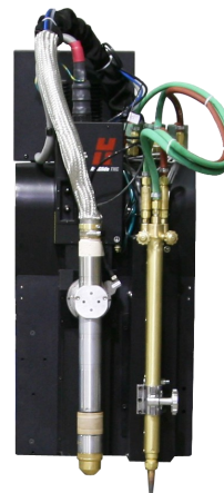
Challenger DSD Master Carriage Equipped with Hypertherm HPR-260 torch, ArcGlide THC with collision sensor, and Oxy-Fuel Torch
