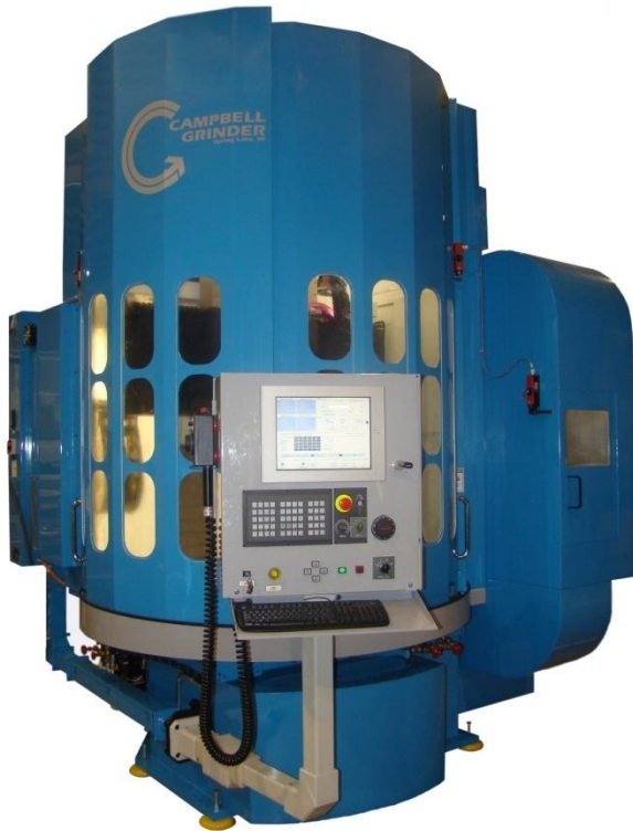
750 Machine with Optional Tool and Coolant Nozzle Changer
