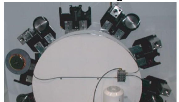
Inside look at Tool and Coolant Nozzle Changer
