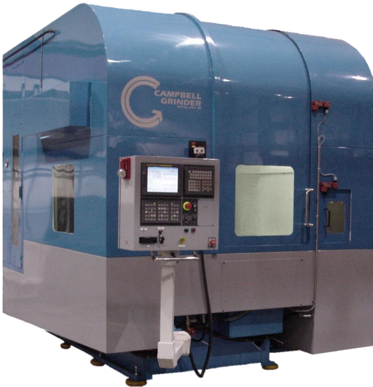
930 Machine with Optional Tool and Coolant Nozzle Changer
