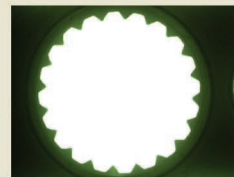
Two times broached component - Not OK
