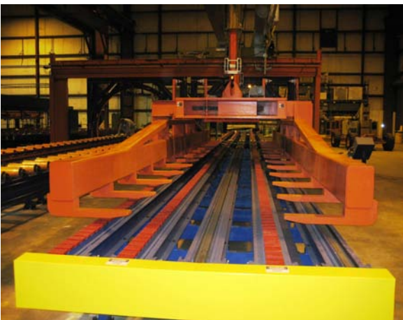
Bushman recently designed this sheet lifter and crane system for a steel and aluminum blanking company. This customer was adding plastic wrapping as a new value-added service. Bushman's heavy duty, motorized sheet lifter picks up 30,000 pound plastic wrapped stacks from a conveyor and puts them on a shipping pallet. This single lifter can safely pick up a wide range of sheet lengths and widths. The lifter has 14 lifting forks on each side, spaced to clear the conveyor rollers, helping to reduce the potential for product damage.
