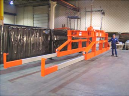
25,000 pound capacity sheet lifter with telescoping carrying arms. Four leg extensions can be manually extended to 40 feet overall length.
