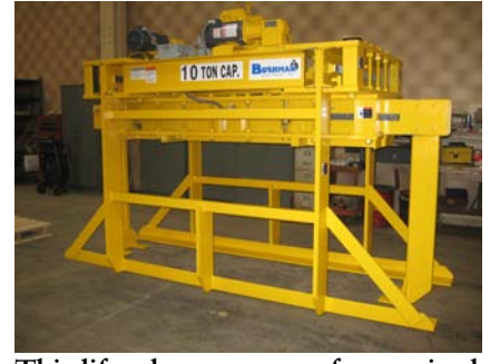
This lifter has two sets of motorized legs to secure the sheet stacks on all four sides.
