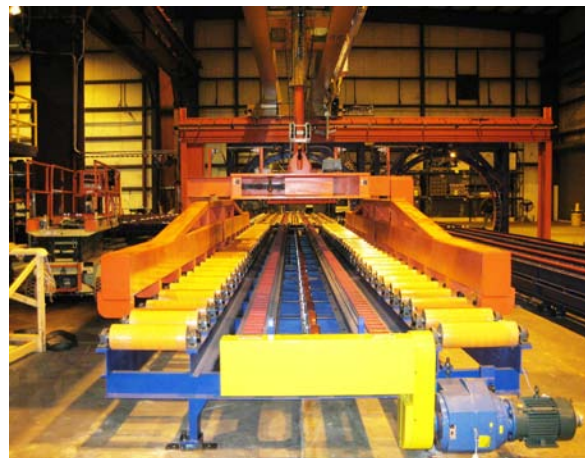
Bushman recently designed this sheet lifter and crane system for a steel and aluminum blanking company. This customer was adding plastic wrapping as a new value-added service. Bushman's heavy duty, motorized sheet lifter picks up 30,000 pound plastic wrapped stacks from a conveyor and puts them on a shipping pallet. This single lifter can safely pick up a wide range of sheet lengths and widths. The lifter has 14 lifting forks on each side, spaced to clear the conveyor rollers, helping to reduce the potential for product damage.
