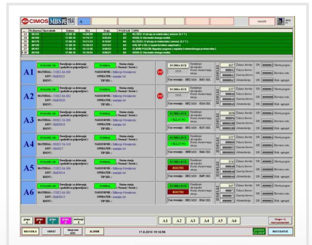
Cell Management module (CM): for monitoring every machine in a cell and provides real time data about material designation, blade identification and operator identification.
