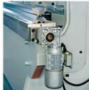
RV减速电机工作台面补偿 RV reducer motor working table compensation
