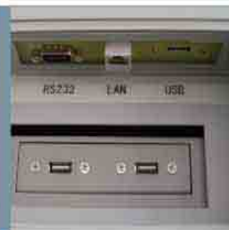
Data exchange ports
