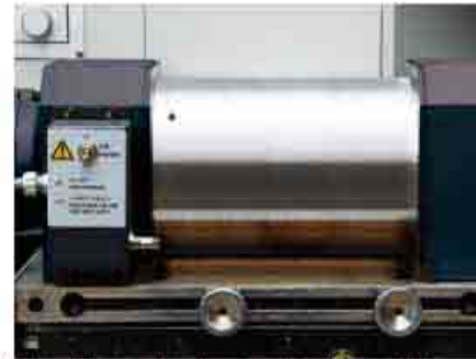
Limit switch on wire drum mechanism, and the surface of wire drum through special treatment in order to increase the life-span
