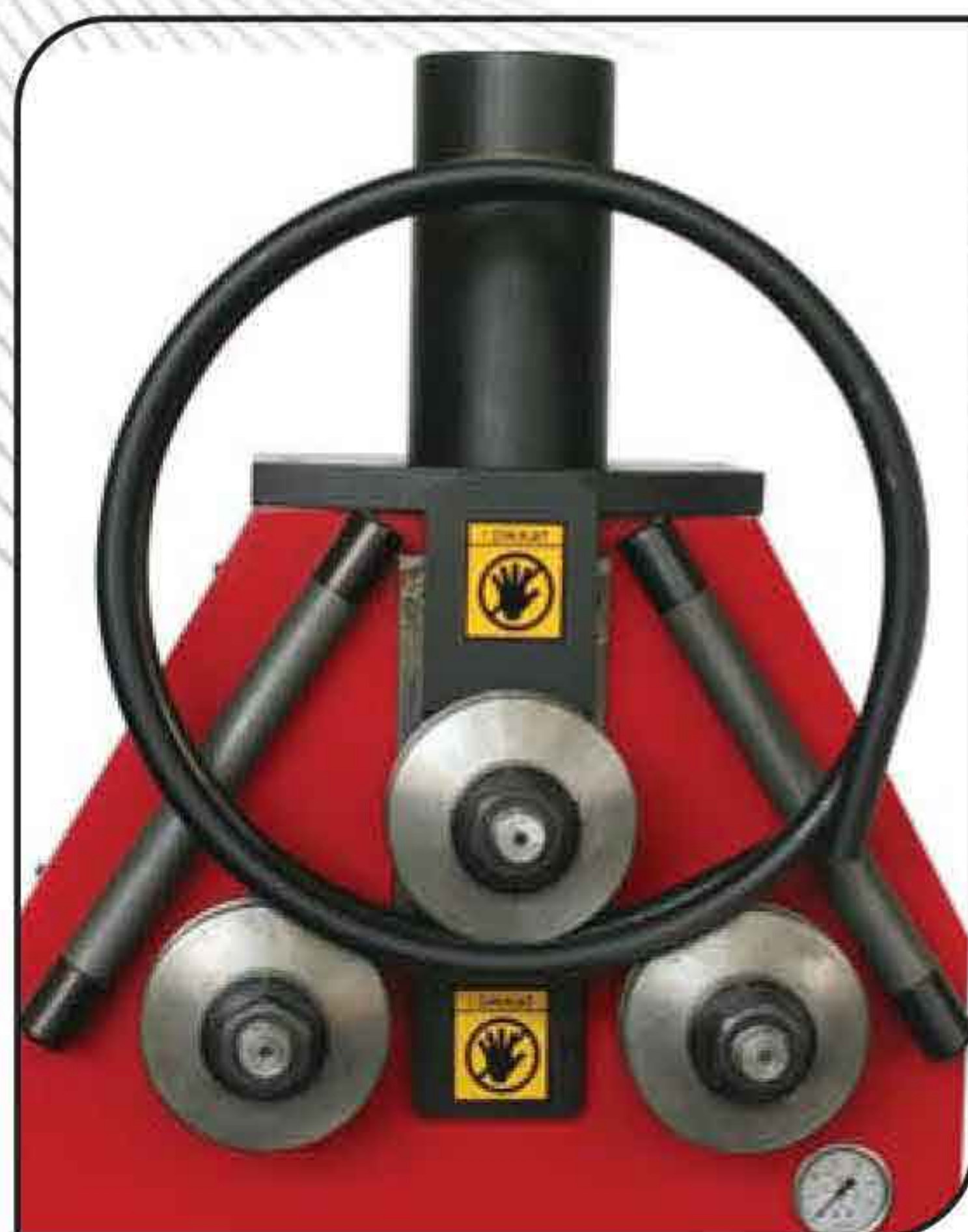
Boru Kıvrma Pipe Bending
