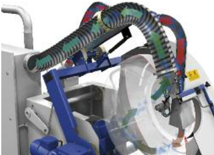
Inlet and exhaust air system; red arrow: heated inlet air, green arrow: exhaust air
