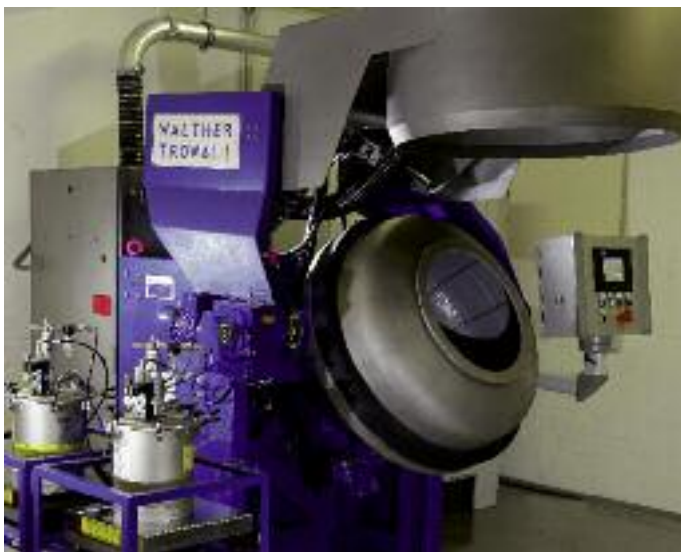
Rotamat R 90 C with opened cover
