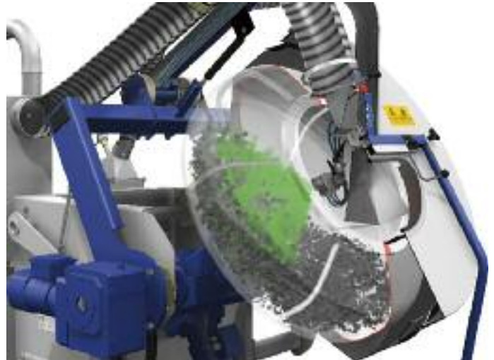
Coating process in a Rotamat machine
