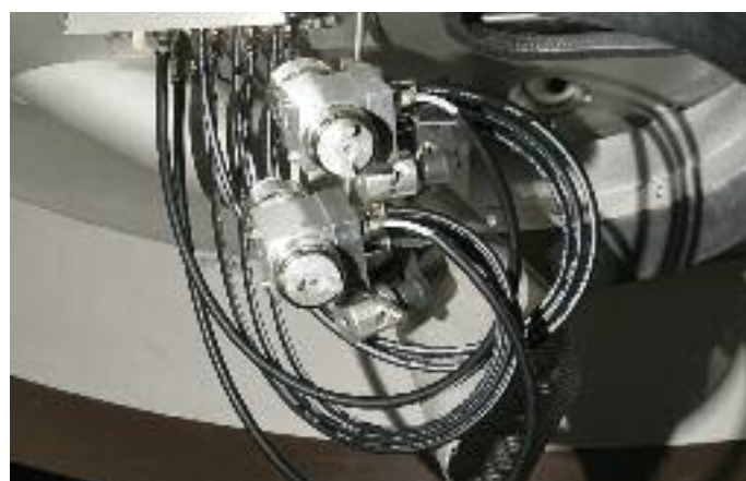
Optional second automatic spraying nozzle assembly
