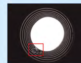
360° 內螺牙牙傷 360° Internal Thread Damage
