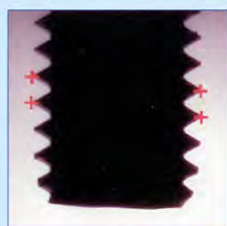
搓牙不良/牙品質 Thread bevel
