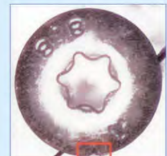
頭上裂痕 Head Crack
