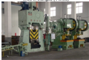
上海汽车连杆CHK31.5kJ-63kJ 2条模锻线 CHK31.5kJ-CHK63kJ connecting rod forging line in Shanghai (2 lines)
