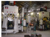
越南工具CHK31.5kJ-CHK50kJ 2条模锻线 CHK31.5kJ-CHK50kJ hand tools forging lines in Vietnam (2 lines)
