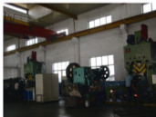
景县叉车零件CHK25kJ-CHK31.5kJ 4条模锻线 CHK25kJ-CHK31.5kJ forklift part forging lines in Jingxian (4 lines)
