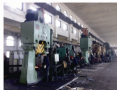
山东威力工具CHK25kJ-CHK100kJ 12条模锻线 CHK25kJ-CHK100kJ hand tools forging lines in Shandong Maxpower Tool Group (12 lines)
