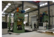
美国史丹利工具CHK31.5kJ-CHK50kJ 2条模锻线 CHK31.5kJ-CHK50kJ hand tool forging lines in Stanley (2 lines)
