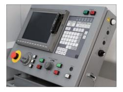
Latest high speed CNC unit Start-up time, screen switching and processing times are considerably shorter. "Cincom Control" is utilized to further reduce cycle times.
