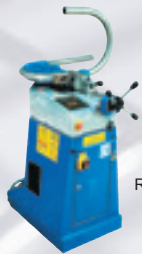
SB48 Super Bender® Capacity 2" tube or 1½" Sch. 40 Max. CLR 8½" Touchpad programming 120V 1ph standard (3ph available)
