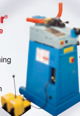
030 Mega Bender® Capacity 3" tube or 2½" Sch. 10 Max. CLR 15" Touchpad programming Mandrel ready 220V 1ph or 220 - 440V 3ph
