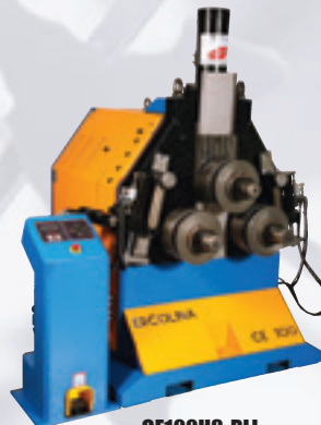
CE100H3-RLI (Hydraulic) 4" Sch. 40 pipe capacity 4" angle iron capacity 220V or 440V 3ph
