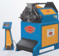
CE50H3 (Hydraulic) 2½" Sch. 40 pipe capacity 2½" angle iron capacity 220V or 440V 3ph
