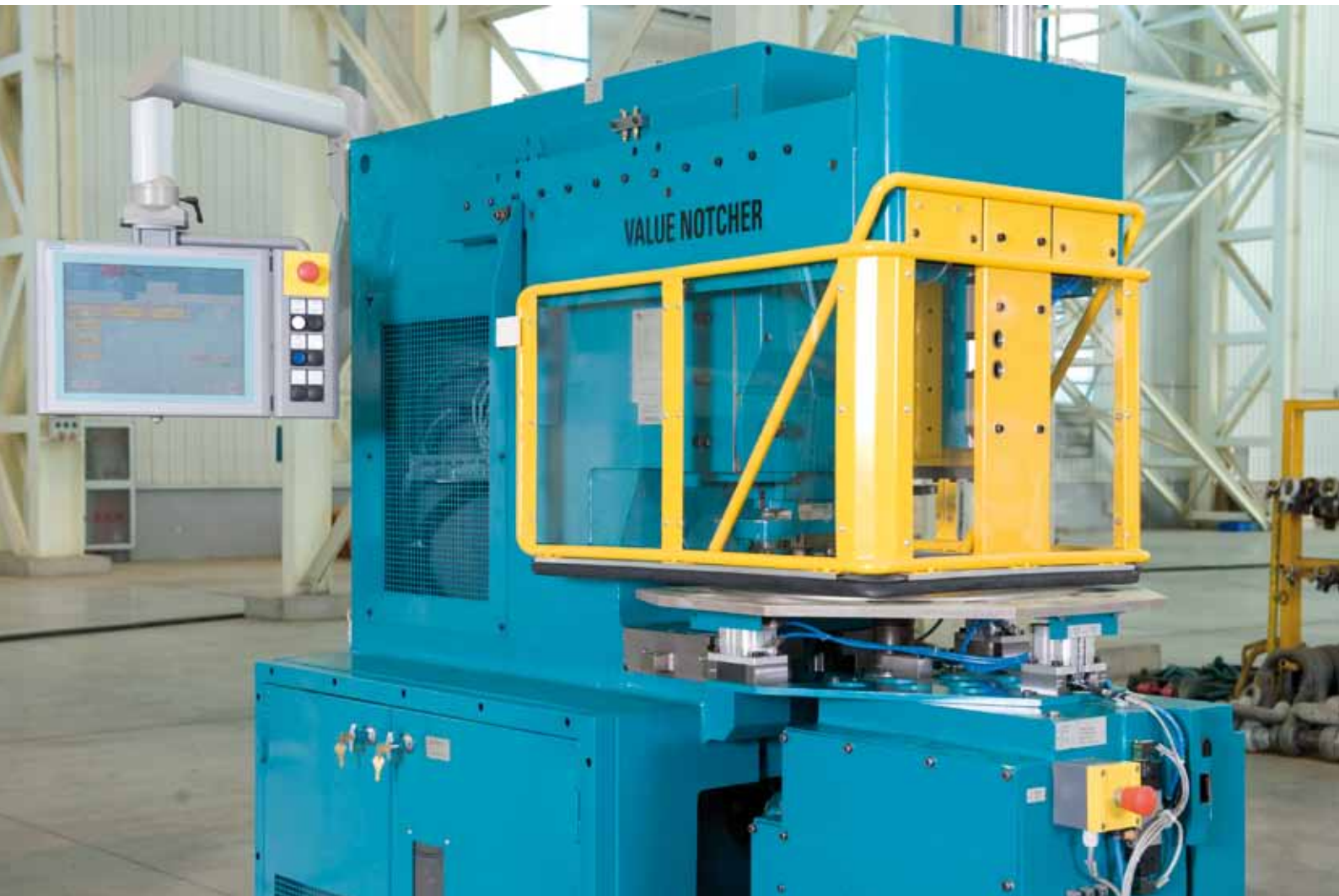
Value Notcher for the cost-effective manufacturing of electric motor lamination
