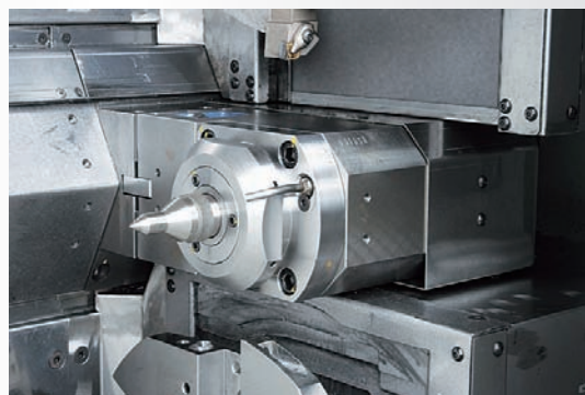
Tail stock - Programmable 350mm long stroke.
