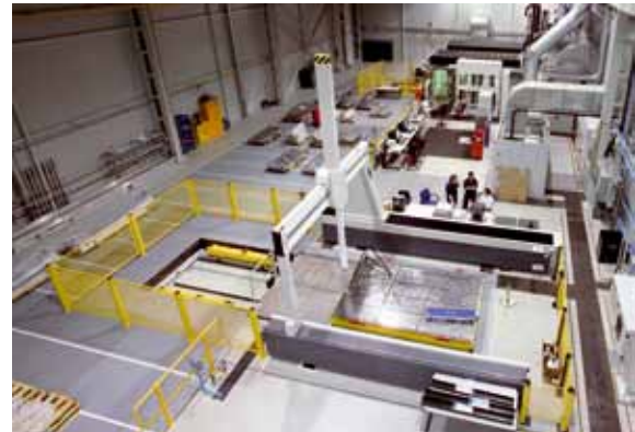
LK V-R twin-rail mounted bridge style CMM
