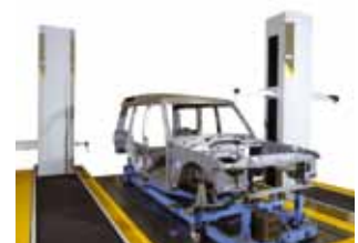
LK H-R dual column horizontal arm CMM
