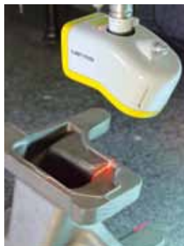
Scanning of casting
