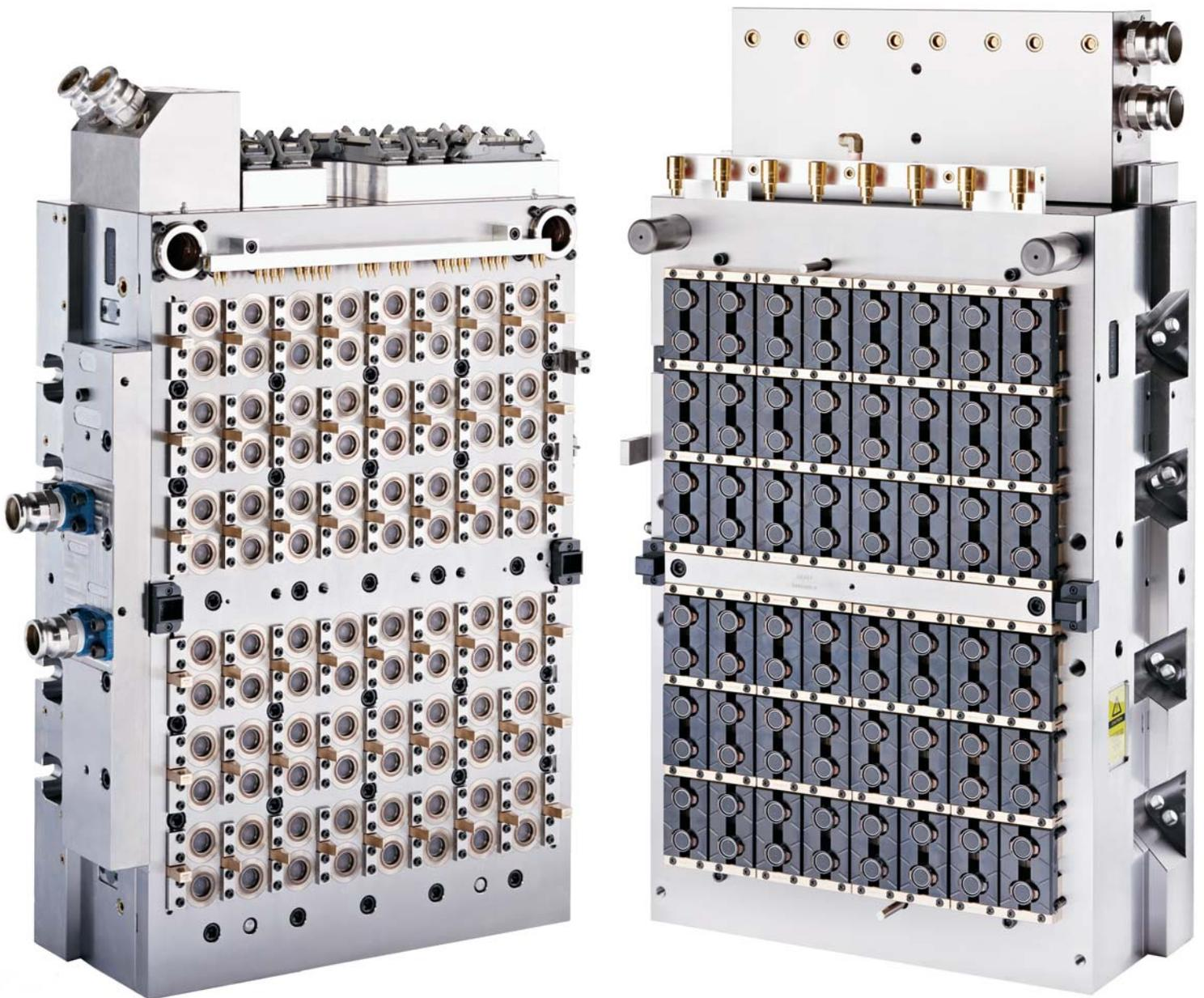
HyCAP features a new mold concept that offers cycle time improvements and quick and easy maintenance to maximize uptime.
