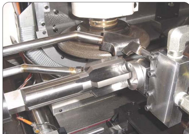
Shown: Fluting M56 Tap from Solid
