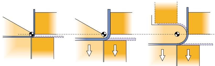
Automatic folding beam and lower beam adjustment: indispensable for perfect radii, precision parts and longer machine life
