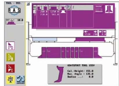
The setup instruction displays which tool segments are required for the length of the part. This information is available for the upper beam, the folding beam and the lower beam. For easy setup, the Touch&More graphically displays the tool shape.
