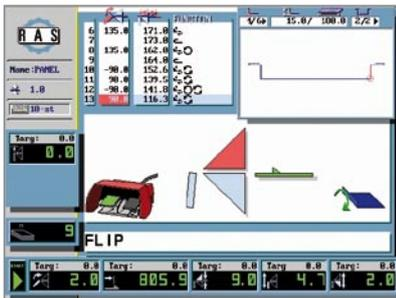
After the program is started, the graphic shows the operator which foot pedal he needs to press. Operator instructions such as „Flip“ or „Paint up“ allow even inexperienced operators to produce perfect parts.
