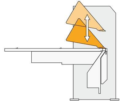
Programmable upper beam position during clamping and unclamping
