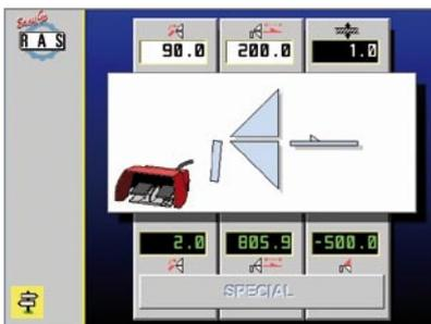
If someone operates the machine occasionally, he can use the EasyGo operation. Simply enter an angle, a backstop dimension and the material thickness and you are ready to go. If you want to bend “by eye” just press the push buttons in the Special menu and start each machine movement separately.
