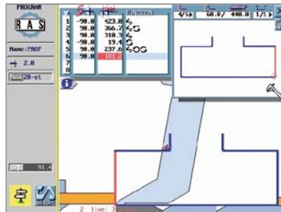
If a collision has been analyzed, the control displays this situation graphically. Technology tables consider material springback. The calculated blank dimensions are automatically corrected by the bend allowance, used for the radii.
