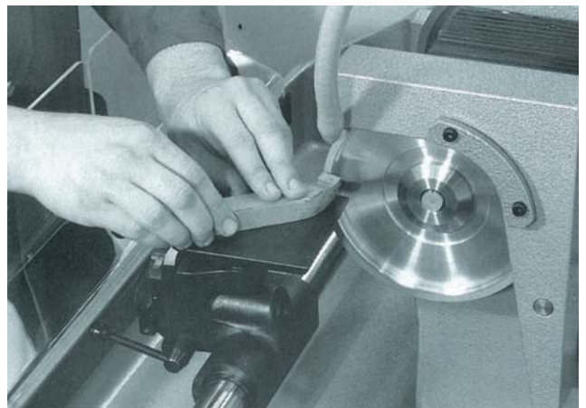
Off-hand radius grinding. Tool on grinding table, item 4.01.73.00
