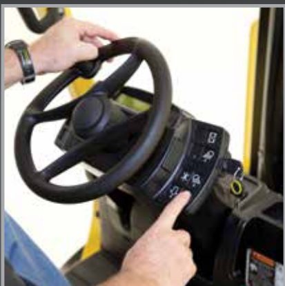
Infinitely adjustable steer column with spinner knob and integrated dashboard display
