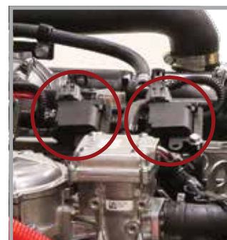
Coil over plug ignition design
