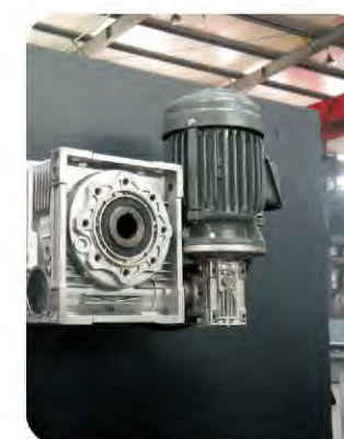
Automatic blade adjustment 刀片间隙自动调整机构
