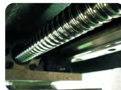
Ball screw and linear guide 直线导轨加滚珠丝杆机构
