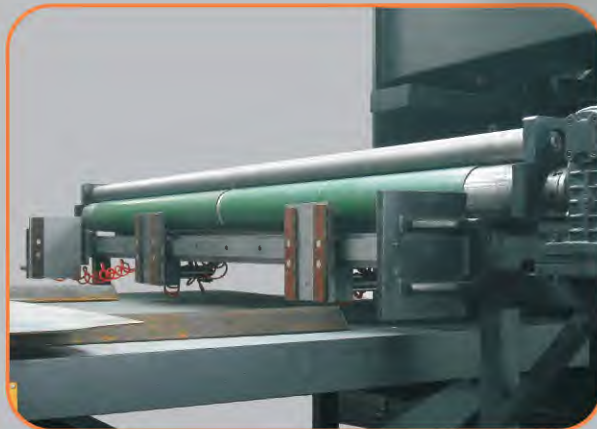
Installation of piling plate 板料码垛机构
