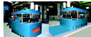
Φ21-Φ114mm 水压试验机 Φ21-Φ114mm Four workstation Hydraulic tester
