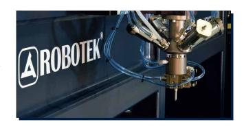
With the variations of accessories and pumps, the mixing head output capacity ranges from 0.3 to 100 g/s with a dosing accuracy of +/– 1%. Custom-ised mixer designs are also available. Material components from liquid to high viscous polymeric reactive materials being dosed in the mixing head are always homogeneous and equally conditioned in correct mixing ratio. By these features, optimized production process is successfully achieved and broad range of applications is easily covered.
