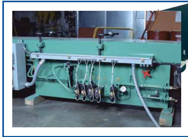
Outside hydraulics with provide ease of maintenance.
