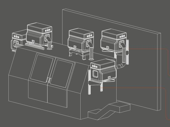
If there is no space on top of the machine tool, all GREEN LINE oil mist separators can be installed on a wall mount.
