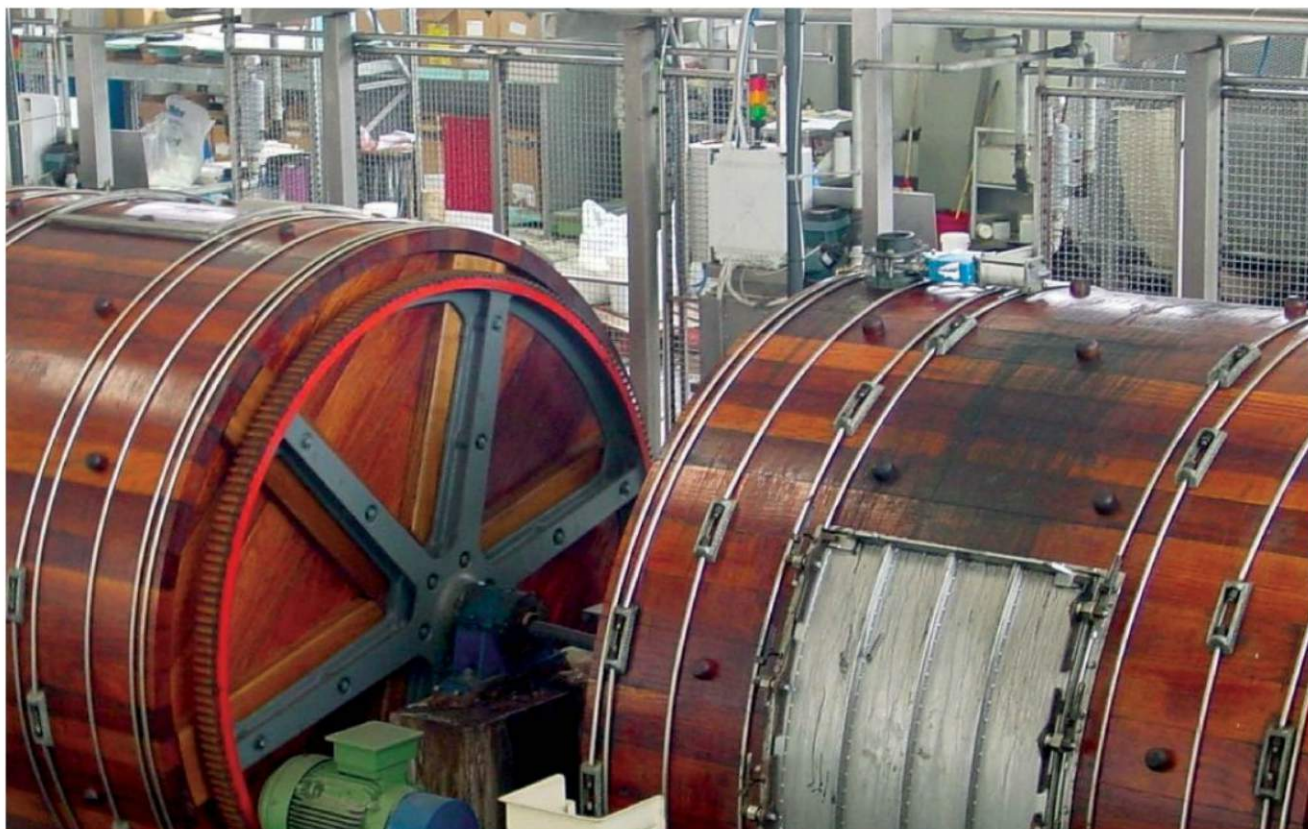
Horween Leathers (Chicago, IL) must use wood tanning drums like these, which come in pieces in order to fit them into their 1905 building.
