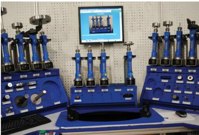
An ergonomic gauge table layout incorporating 48 Marposs iWave wireless bore gauges has enabled a leading North American automotive supplier to reduce by one-half the time needed for audit inspection of two transmission components.
