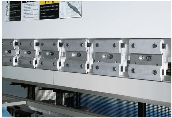
Available Quick Lever Clamping allows tool-less upper punch changes while maintaining individual adjustability
