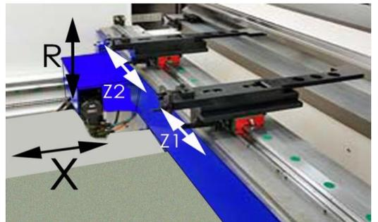
Extra Backgauge fingers available. Customer choice of finger shape. All fingers have hardened replaceable inserts at tip. Tips flip up to avoid damage to gauge or workpiece.
