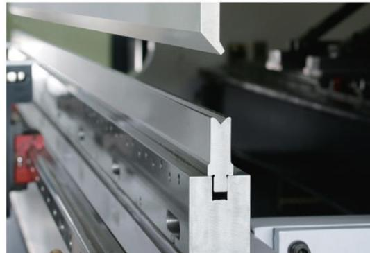
Available Double-V lower tooling (Amada-style) allows a close return in one direction and changing of opening by rotating the lower die upon its tongued support. Front-to-back adjustable and provides some front support for small parts if the rear opening is in use.
