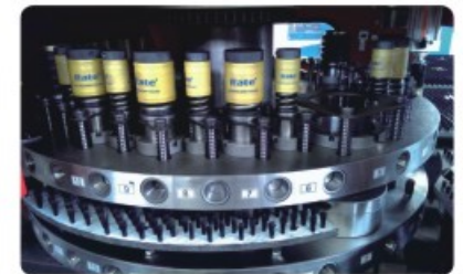
镶套式轮盘，标准模具 Turret station with sleeves, standard tools
