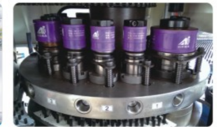
镶套式轮盘，标准模具 Turret station with sleeves, standard tools
