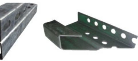
槽钢冲孔 Channel punching
