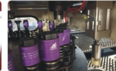
独特夹钳避让，无死区加工 Clamp automatic avoids function No processing dead area on sheet metal
