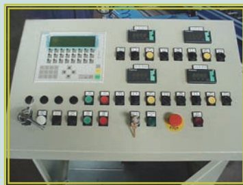
Electronic control by PLC
