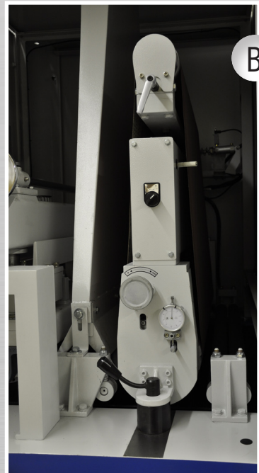
Picture B: Contact drum sanding head with cam adjustable head to accommodate varying belt thicknesses
