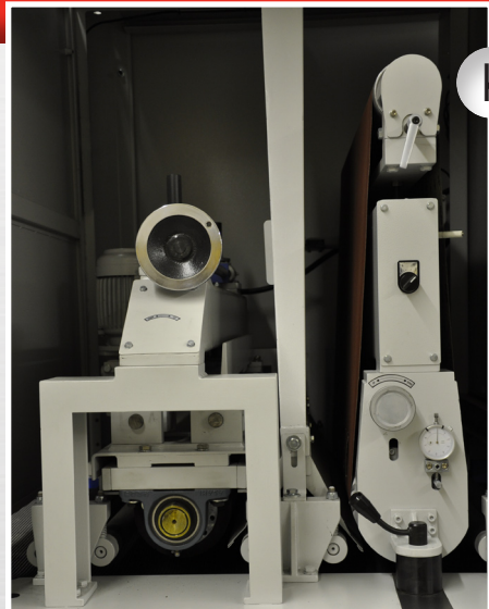
Picture A: Barrel brush head with variable speed and oscillation
