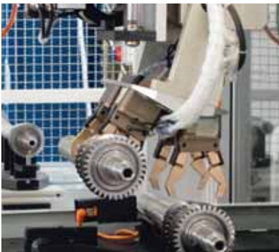
Gantry loader with double gripper
