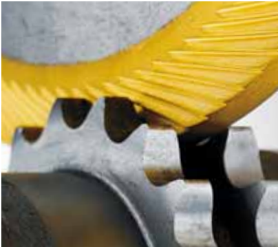
Deburring of a chain sprocket gears
