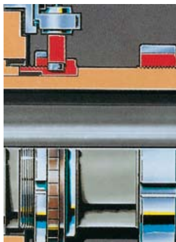
C-axis with hollow shaft encoder for maximum positioning accuracy considerably enhances the range of application.
