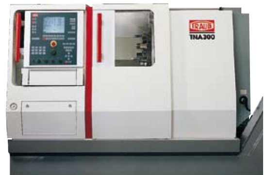
Safety envelope with state-of-art design and safety windows of polycarbonat and glass laminate.
