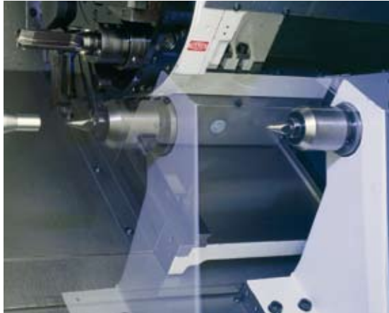
The tailstock offers a large automatically adjustable working range.
