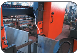
33- PROXIMITY SWITCH FOR SENSING BLADE SLIPPAGE
