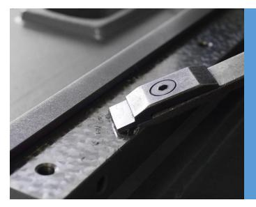
Star and Seibu machine surfaces are hand scraped by skilled craftsmen to provide accuracy and stability. Fanuc controls provide the most advanced, reliable CNC controls on the market today.
