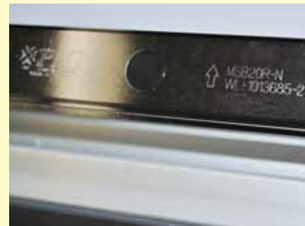
Precision linear rails and bearings provide smooth play-free motion
