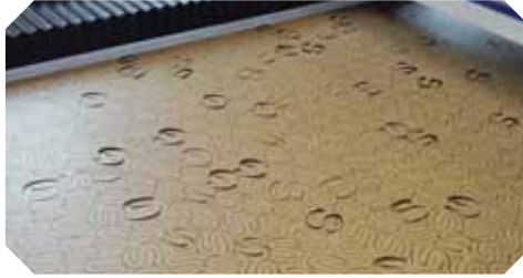
Techno CO2 Laser 4896 | 150 Watt with Cast Acrylic Sheet
