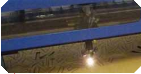
Techno CO2 Laser 4896 | 150 Watt with Cast Acrylic Sheet
