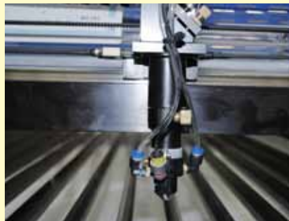
State-of-the-art CO2 laser design
