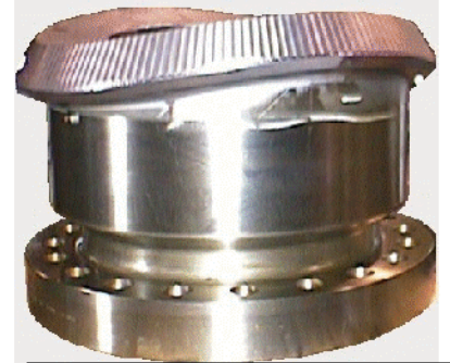
Heavy Self-Reinforced Nozzle mad to suit side intrusion into Vessel (for project)
