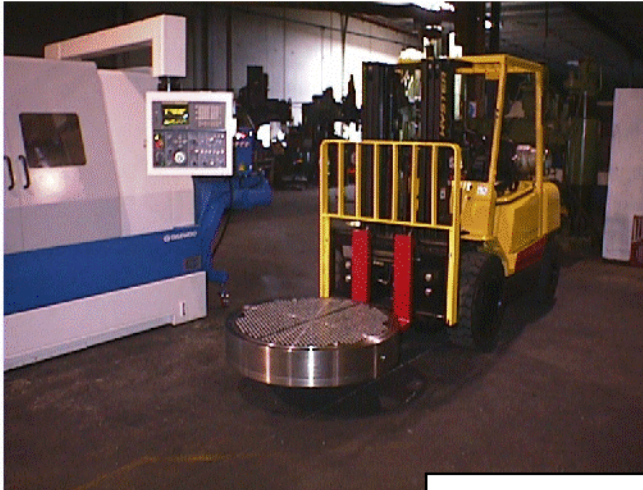
Large Tubeplate 210 Thick 1092 Holes in High Yield Material
