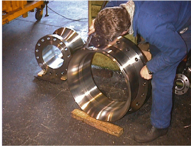
Heavy Self-Reinforced Nozzle mad to suit side intrusion into Vessel (for project)
