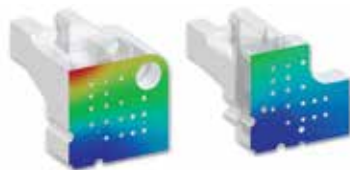
Left, uneven pressure. Right, improved uniform clamping force.
